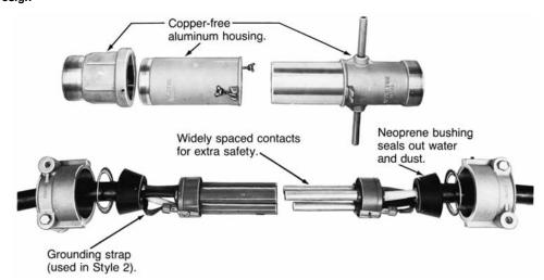
**Energized contacts** deeply recessed to reduce danger of accidental touching, minimize possibility of exposed arcs. Insulator quenches arcing, and is resistant to abnormal heat and to fire.
