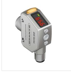
Q4X Series: Laser Adjustable Field Range: 300 mm; Input 10-30 V dc Outputs: Bipolar: 1 NPN; 1 PNP Connection: Euro M12 5-Pin Integral Connector Part Number: 94118
