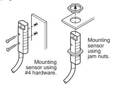
A second mounting method is to use #4 hardware in the 0.125 inch diameter mounting holes in the flat sides of the sensor. This is ideal for mounting the Comet against a wall, piece of equipment, rail, mounting bracket, etc.
