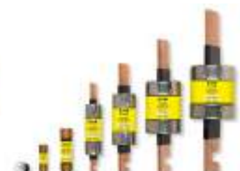
LPN-RK — Class RK1, 250 V, 300 kA IR up to 600 A
