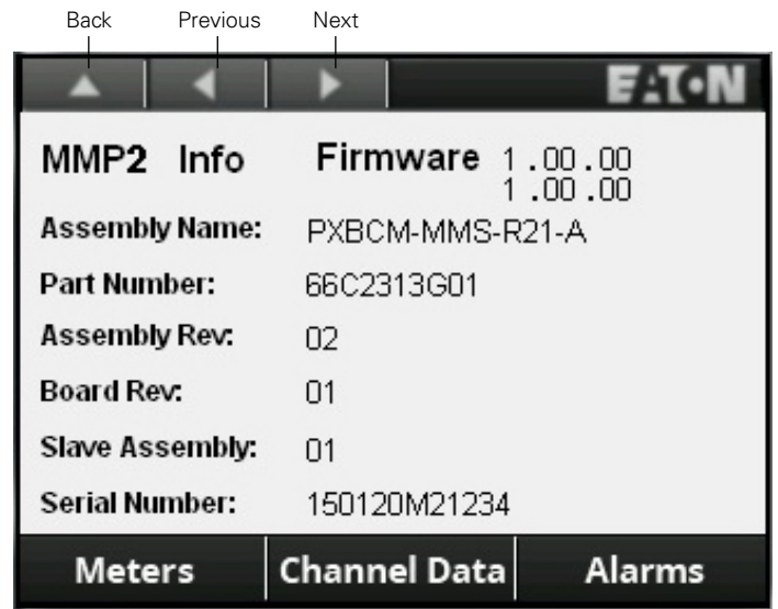
Figure 5. Meter module information.
