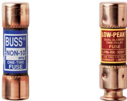
In the above illustration, the fuse on the right has a grooved ring in one ferrule, providing the rejection feature of the Class R fuse in contrast to the lower interrupting rating, non-rejection type.
