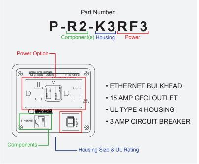
GracePorts® are fully customizable panel interface connectors that allow workers to access control panels safely and conveniently through closed doors therby reducing the risk of arc flash. These ports can be conveniently installed on the cabinet door without voiding the UL rating of the cabinet. They can be used to program PLCs and Variable Frequency Drives (VFDs), machine interfaces, connecting laptop from outside to access and program control components.
