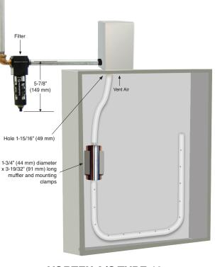
VORTEX A/C TYPE 12 (SHOWN TOP MOUNTED ON CUSTOMER'S ENCLOSURE)
