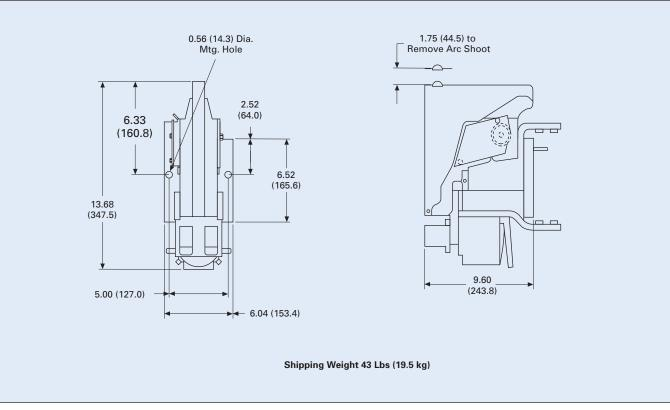
D-Contactor Approximate Dimensions in Inches (mm), and Shipping Weight
