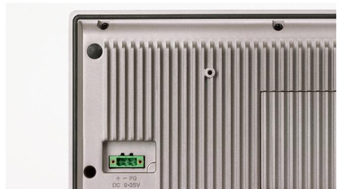
Figure 10. Power port connection.
