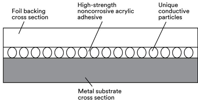
**Figure 2** Embossed Backing with “Through-the-Adhesive” Contact
