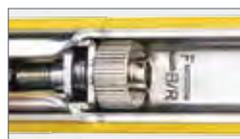
Connector markings for quick adjustments.
