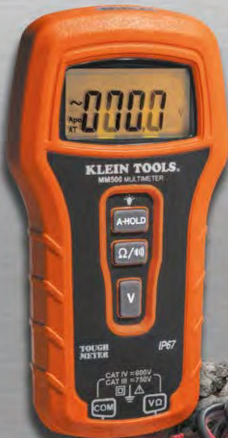
The **Klein Tools Auto Ranging Multimeter** measures AC/DC voltage, resistance and continuity.
