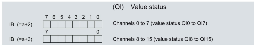
Figure 4-1 Address space for configuration as 16-channel DI 16x24...125VUC HF QI with value status
