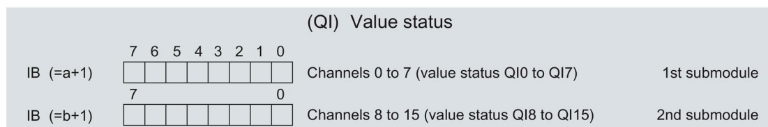
Figure 4-2 Address space for configuration as 2 x 8-channel DI 16x24...125VUC HF S QI
