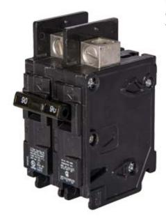
Siemens Low Voltage Molded Case Circuit Breakers General Purpose MCCBs - Type BQ, 2-Pole, 120/240VAC are Circuit Protection Molded Case Circuit Breakers. 2-Pole Common-Trip circuit breaker type BQ. Rated 120/240V (040A) (AIR 10 kA). Special features: Load side lugs are included.
