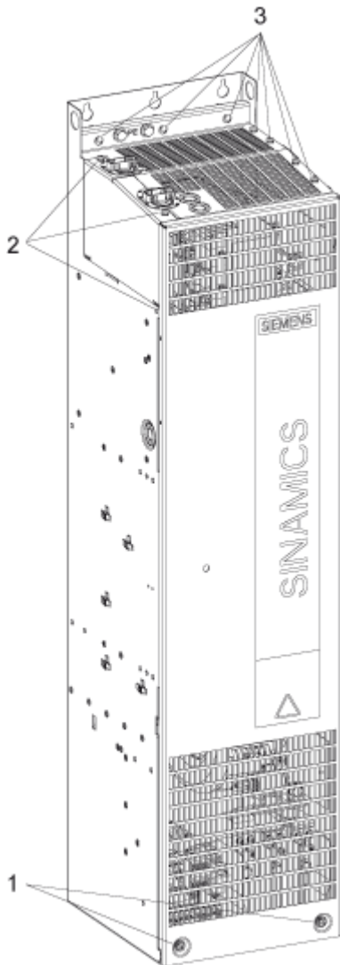
Figure 6-6 Installing the Braking Module in a Power Module, frame size FX – steps 1 - 3
