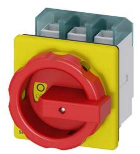
SENTRON, 3LD switch disconnector, EMERGENCY-STOP switch, 3-pole, lu:100 A, Operational power / at AC-23 A at 400 V: 37 kW, front- mounted, rotary operating mechanism, red/yellow, 4-hole mounting of the handle
