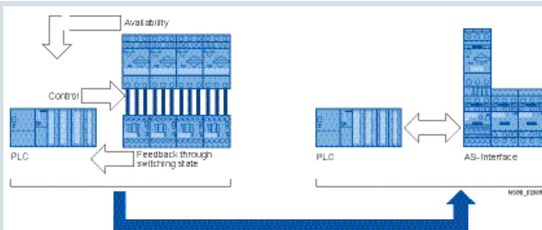
Signal transmission through AS-Interface
