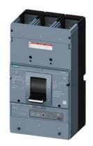
circuit breaker 3VA6 UL frame 1200 breaking capacity class H 65kA @ 480 V 3-pole, line protection ETU320, LI, In=1200A overload protection Ir=500A - 1200A short circuit protection Ii=1,5-10 x In w/o connection
