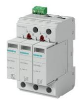
Surge arrester, Type 2, pluggable protective modules, UC 750V AC, 3-pole, for 4-wire networks (L1, L2, L3, pen), with remote signaling
