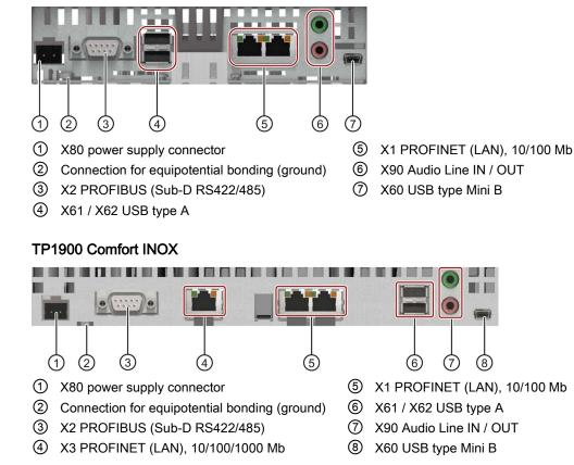
Use the X1 or X60 interface to connect a configuration PC. Use the X61 / X62 interfaces to connect peripheral devices such as a printer or keyboard. Use the X90 interface to connect a loudspeaker.
