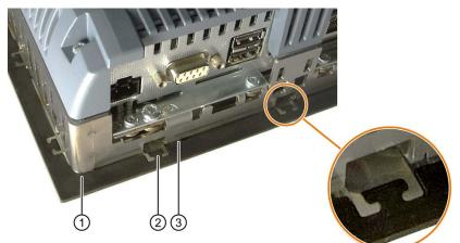
2. Place the mounting gasket as shown on the stainless steel face.
