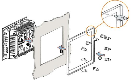
2. Turn the setscrew of each mounting clip until a slight clamping force is perceptible.
