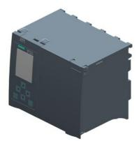
SIMATIC S7-1500, CPU 1518-4 PN/DP MFP, central processing unit with C/C++ Runtime pre-installed, 6 MB work memory for program and 60 MB for data, 1st interface: PROFINET IRT with 2-port switch, 2nd interface: PROFINET RT, 3rd interface: Ethernet, 4th interface: PROFIBUS, 1 ns bit performance, SIMATIC Memory Card (min. 2 GB) required
