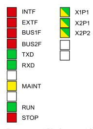
Figure 4-1 LEDs front panel CP 443-1 Advanced
