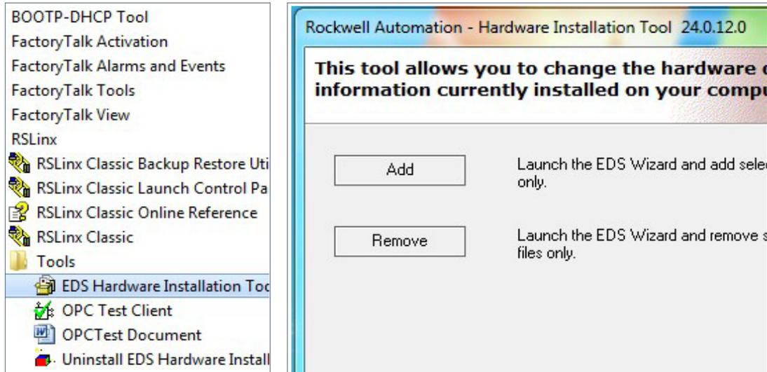
Let's start off by registering the EATON EDS files into RSLINX with the EDS Wizard.
