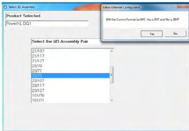
**STEP 5:** Select the appropriate DG1 I/O Assembly Pair as previously completed in the RS5K project; **23/73** in this example.
