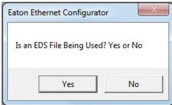
**STEP 13:** The EIP-Assist tool will loop back to the original prompt of whether an EDS is to be utilized. Referring back to the second Eaton product that was added, *the EDS file was indeed utilized.*
