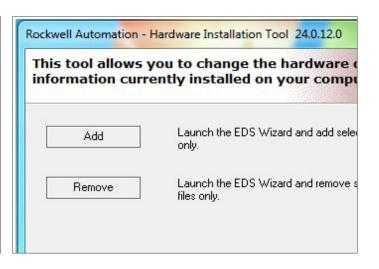
Let's start off by registering the EATON EDS files into RSLINX with the EDS Wizard.
