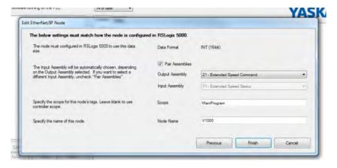
STEP 8: Select the I/O Assembly pair that was used in the RS5K project (21-71)
